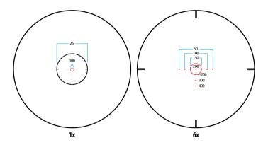
The G3F1624 Scope is equipped with a Type-C reticle designed with set marks for estimating distance and for holdover correction. *1 MOA (Minute of Angle) = approx. 1 inch @ 100 yards away.*
