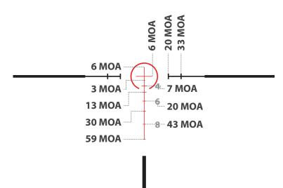
The scope uses a first focal plane reticle, meaning the size of the reticle relative to the target image stays consistent across different magnification settings. This is useful because the ranging information from the reticle hashmarks remains constant regardless of magnification setting, allowing for faster, more convenient range estimation and holdover correction.
