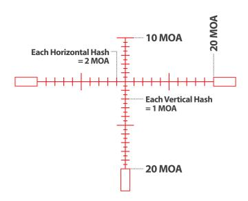
The scope uses a first focal plane reticle, meaning the size of the reticle relative to the target image stays consistent across different magnification settings. This is useful because the ranging information from the reticle hashmarks remains constant regardless of magnification setting, allowing for faster, more convenient range estimation and holdover correction.
