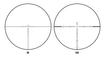
The G2-FFPS41650 Scope is equipped with a Type H FFP reticle designed with set hashmarks for estimating distance and for holdover correction. 1 MOA (Minute of Angle) = approx. 1 inch @ 100 yards away.
