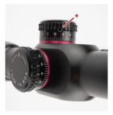
The windage and elevation dials have numbered markings at the base and can be reset to zero for a simpler point of reference. To reset the turrets to zero, simply unscrew the hex screw on the sides of the turret. Rotate the turret to align the "0" with the reference point at the base of the turret, then re-insert the hex screw.
