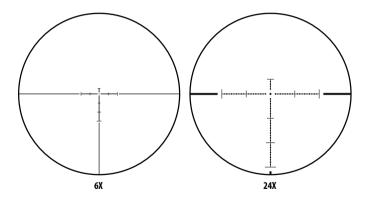
The G2-FFPS62450 Scope is equipped with a Type H FFP reticle designed with set hashmarks for estimating distance and for holdover correction. 1 MOA (Minute of Angle) = approx. 1 inch @ 100 yards away.
