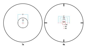
Numbers above the center are an approximate range of yardage for a 18in target. Numbers below the center are an approximate BDC for a 55 grain 5.56 round. The GA1424 Scope is equipped with a Type-C reticle designed with set marks for estimating distance and for holdover correction. *1 MOA (Minute of Angle) = approx. 1 inch @ 100 yards away.*
