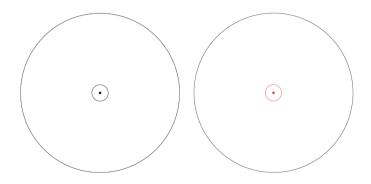
The P332R Scope is equipped with a Circle Dot reticle designed with set hashmarks for estimating distance and for holdover correction. *1 MOA (Minute of Angle) = approx. 1 inch @ 100 yards away.*
