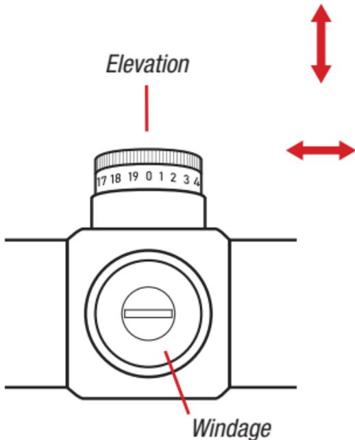
Twist the top dial to adjust the Elevation (80 MOA)
